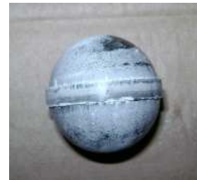
Fig. 7. Collar formed on the spheroid after hydraulic shaping
