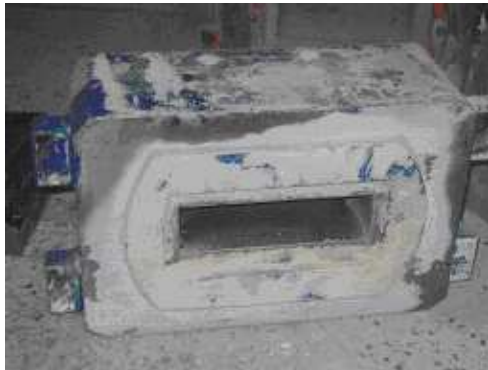
Fig. 8. Die box of alumina bricks for linings
