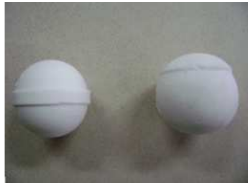
Fig. 11. Shaped and sintered spheroids (left) hydraulic shaping; (right) isostatic shaping
