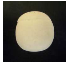
Fig. 6. Sphere produced by isostatic shaping
